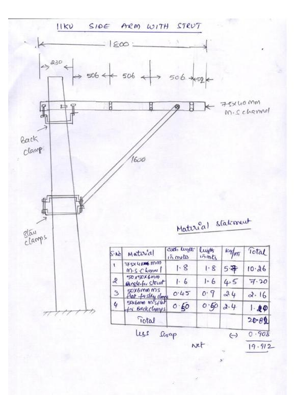
A Tolerance on weight per meter shall be <u>+</u> 2.5% as per IS 1852:1985.
